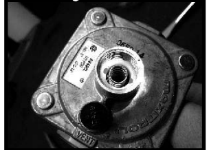
8. To adjust pressure: Remove brass cap & turn white plastic part inside the stem of regulator
