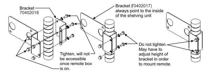
2. Remove screw and washer from remote box. Align the holes of the remote box with those of bracket 70402017. Screw the remote box to bracket 70402017. Once remote box is mounted to bracket, adjust height of the bracket so that the top of the remote box is even with or underneath the bottom of the side shields on the shelving unit (**min. distance 4"** between the bottom of heat strip and top of remote box) and tighten screws.
