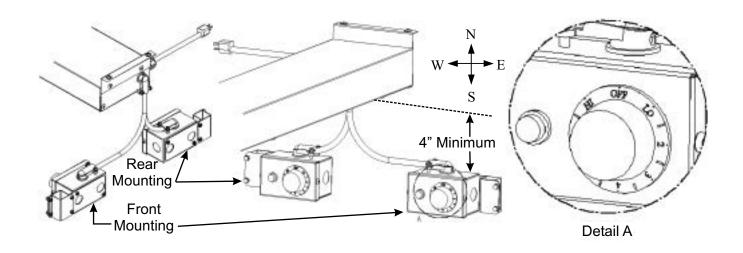
1. Use 88904 (screw), 89056 (washer), and 88921 (nut) to mount bracket. Place bracket (70402017) around shelving pole on the inner side of the shelving unit. Screw bracket (70402018) to bracket (70402017) around shelving pole on the outer side of the shelving unit. The bracket will allow the remote box inner side to align with the front side of the food warmer
