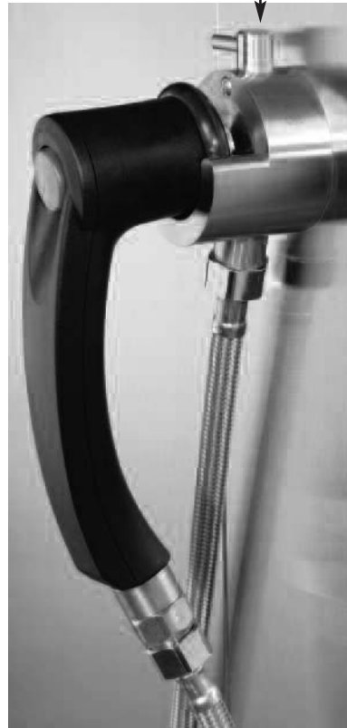
SHUT-OFF VALVE SHOWN IN THE OFF POSITION
