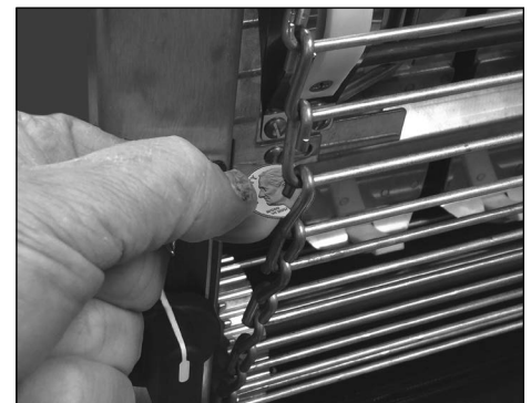
Figure 7. Measuring Conveyor Belt Chain
