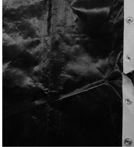
Belt is missing snaps and is damaged. Replace all Belts.
