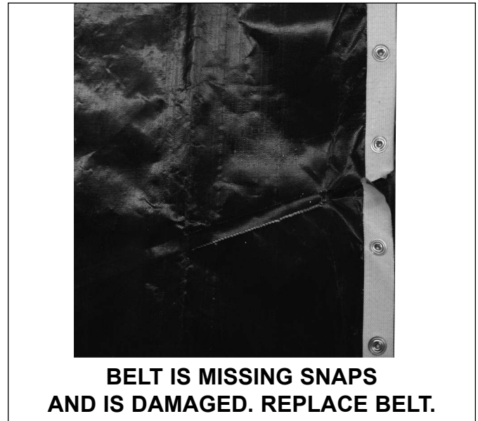
Figure 6. Example of Damaged Belt
