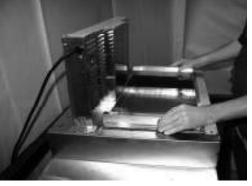
8. Plug electrical cord into power receptacle of the table.
