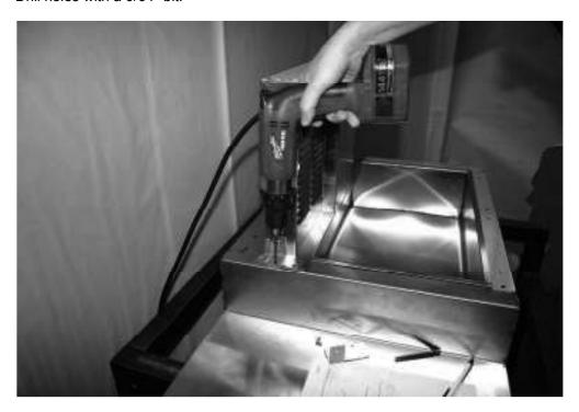
5. Insert and tighten screws provided (SCR008).
