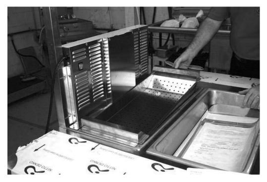
13. Plug electrical cord into power receptacle of the table.
