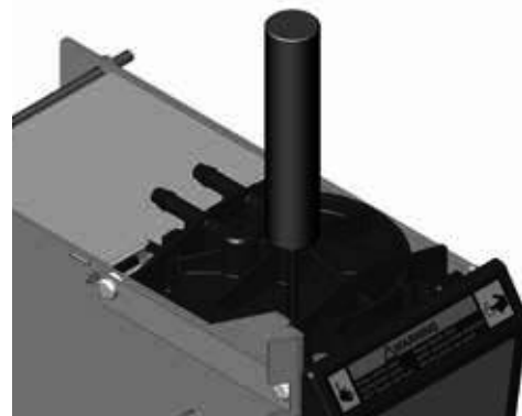
FIG 22-4 Insert alignment tool.
