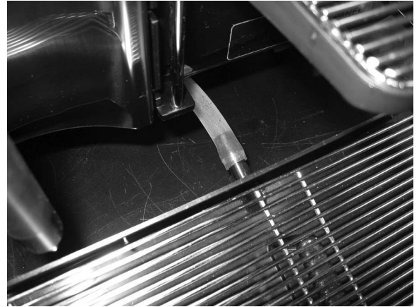
INSTALL DRAIN HOSE AND DRIP TRAY
