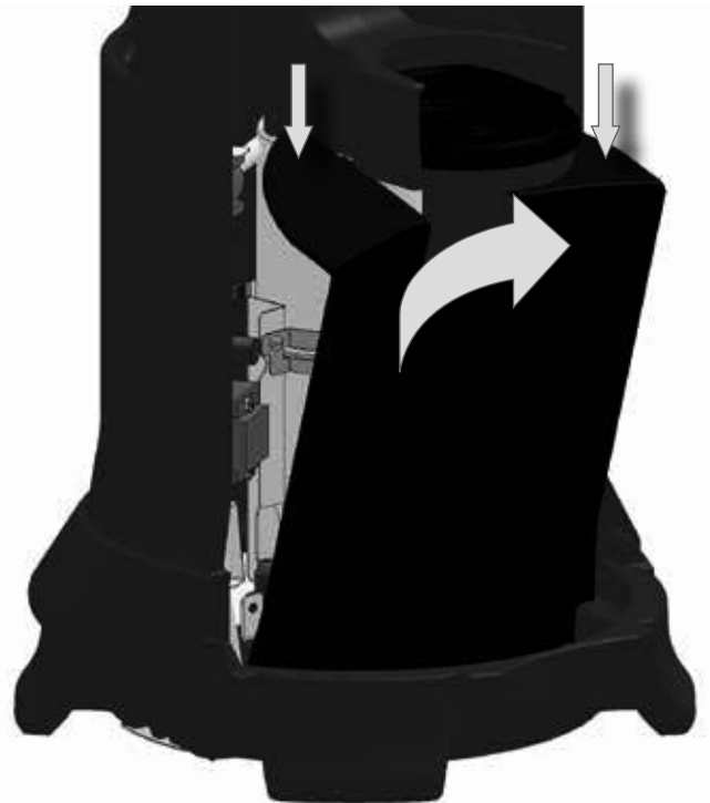
FIG. 10-4 Pull top of panel towards you while pushing down on the side flaps.
