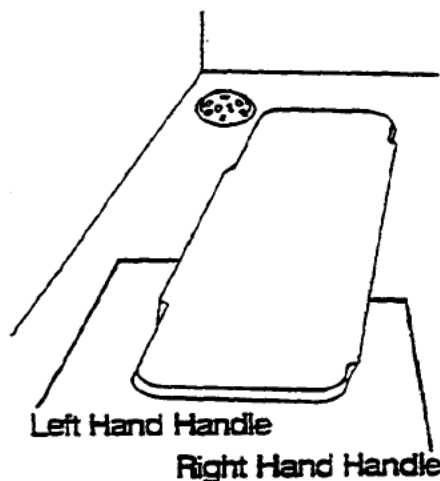
Figure 2-10. Steam Generator Cover in Place
