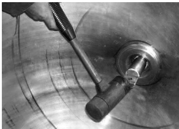
10. Tap shaft back to seat up against retaining ring. 11. Complete reassembly by reinstalling bolt and end cap.
