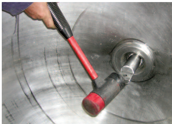
10. Tap shaft back to seat up against retaining ring.
