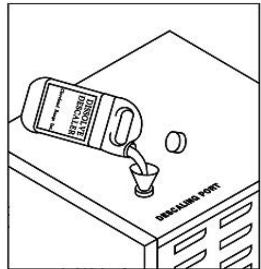
Figure 6-1 Descaling Port Located at Right Rear of the Combi
