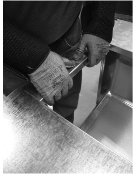
Photo 1. The units should be lifted by the bracing only
