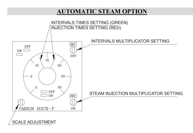
By pushing the GREEN button, the button will light up and the automatic system injection will start. The injection will be done as per the pre-adjustment time on the automatic steam timer. The standard steam timer (white light) will light up during the steam injection. Push the RED button to stop the automatic steam injection and then, the GREEN button will turn off.
