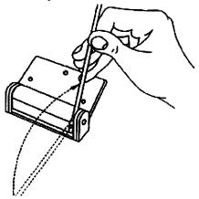
The hinge has been designed so all parts are replaceable. It is usually not necessary to order a complete replacement hinge. The parts list in the back of this manual illustrates and lists all the hinge parts. By only ordering parts that need replacement, maintenance costs can be reduced.
