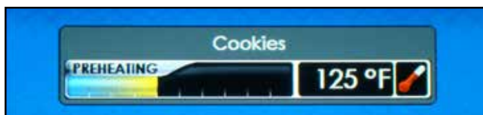
Figure: Oven Recipe Preheat Screen (if under temp. setpoint for bake only recipe; i.e. Cookies):
