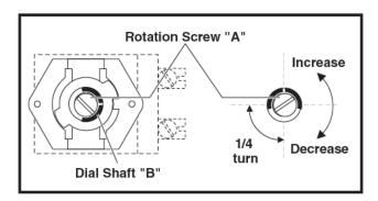
NOTICE: Maximum turn of screw "A" is 1-1/2 turns – clockwise or counter-clockwise.
