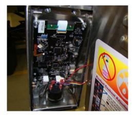
9. Remove the 2 hex screws holding the buzzer using an 11/32" nut driver.
