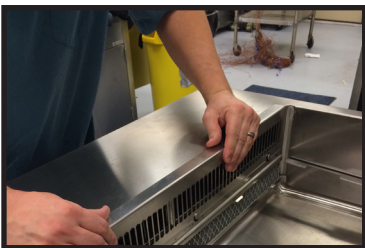
Insert Filter after clean and dry back into position.
