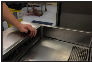
Insert Plenum Return after clean and dry back into position.
