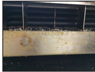
Wipe any debris build up that has accumulated behind the removable filter. CAUTION: This area may be hot.
