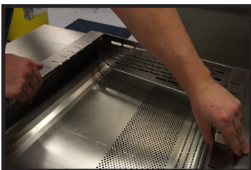
Insert Basket aligning tab and slot after clean and dry back into position.
