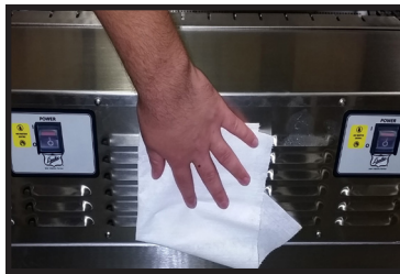
Wipe down the front louvered panel. Ensure no debris accumulation on the louvers as this can degrade the performance of the equipment
