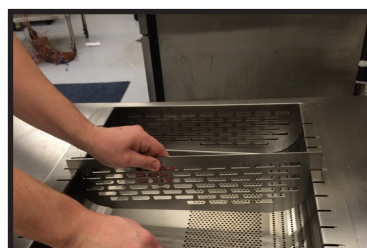
Insert Lane Dividers after clean and dry back into position.
