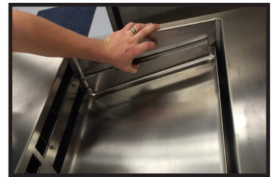
Insert Collection Pan after clean and dry back into position.
