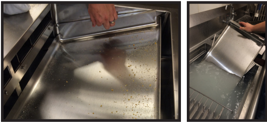
Remove Collection Pan and clean in three compartment sink.
