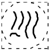
Mixed cycle: superheated steam. Uses the oven chamber heaters and steam generation system at the same time to keep food soft (maximum temperature 482°F)(250°C).
