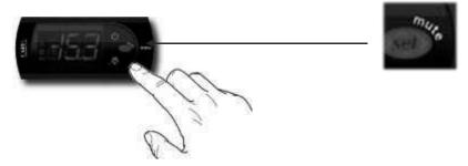
2. Press the up and down arrows to increase or decrease the set temperature. Then press the set button to save the new set point.
