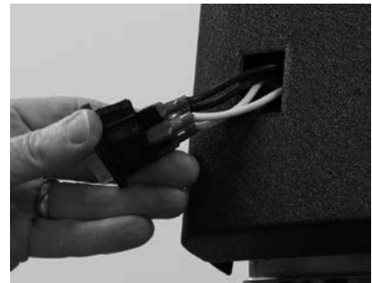
Pull switch out to access terminals.
