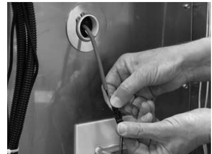
Disconnect Low Product Sensor from harness terminal.
