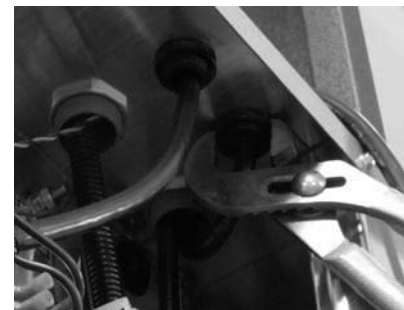
Loosen and remove power cord strain relief nut.
