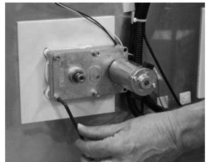
Remove the four motor mounting screws.
