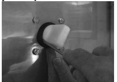
Cut or pry off old shaft gasket and discard.
