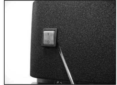
Insert flat screwdriver to release top & bottom locking tabs.
