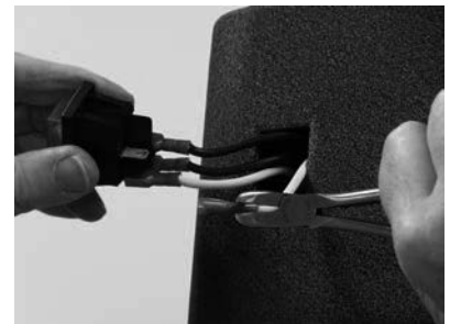
Remove harness connections from four switch terminals.
