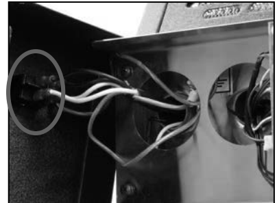
Remove black & white cord leads from Power Switch.
