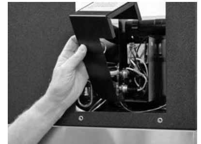
Remove screw & slide up/off relay box cover.
