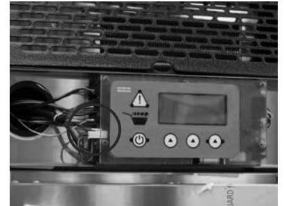
Disconnect 24-volt power lead at Main Control Board [24v].
