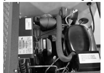
Access the condenser fan motor from open top of compartment.
