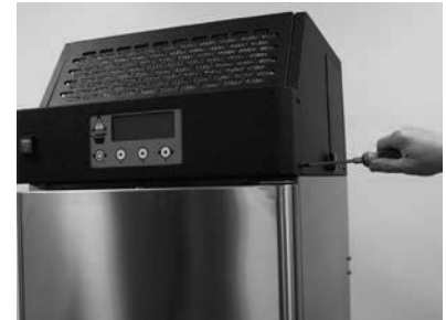
Remove four front control panel cover/bezel screws.
