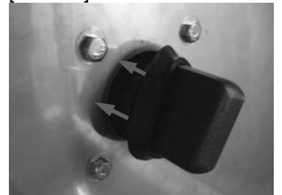
Mount new block using four bolts provided. Press seal over shaft & tight against freezer wall.
