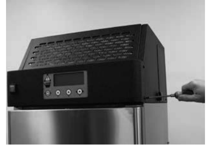
Remove four front control panel cover/bezel screws.
