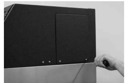
Remove the right side service access panel.
