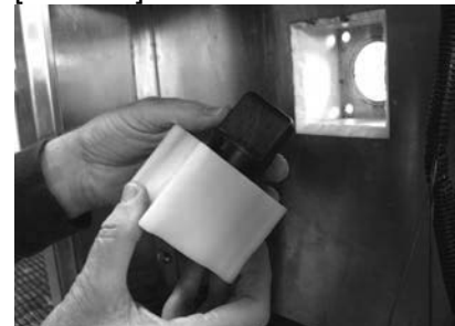
Insert new rotor/motor shaft in contoured rotor block.
