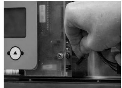
Disconnect TEMP PROBE connector from left control board terminal, pull through to right board & connect to that TEMP PROBE terminal.
