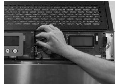
Connect B-B (Slave) to left control board terminal
