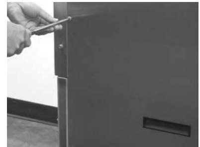
Remove four screws & lift off rear service access panel.
