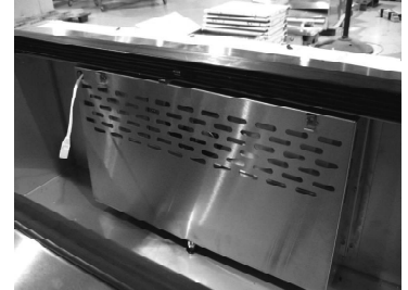
Unplug display light cord and remove four screws that secure evaporator fan cover.
