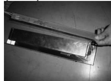
The small flexible heater is attached to the tank bottom by a peel-and-stick adhesive strip.
