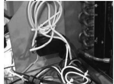
Identify temperature sensor cable. Cut plastic tie securing excess cable and remove that terminal from controller.
