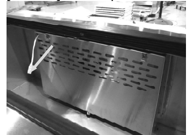
Unplug compartment light from fixture and remove four screws to remove evaporator fan cover.
