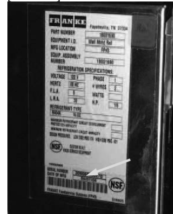
The BBR Unit Serial Number is located adjacent to the Model Number & Data sticker, which is on the left side, when facing unit.
