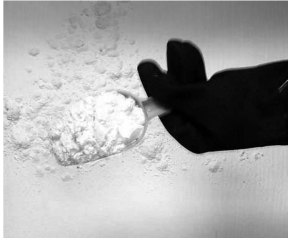
Sprinkle the proper amount of filter powder evenly over the paper.
