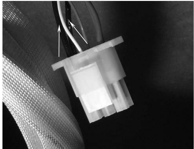
Using a pin-pusher, remove two high-limit wires (arrows) from connector.
