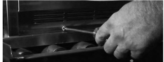
Fig. 1. Removing side panel.
