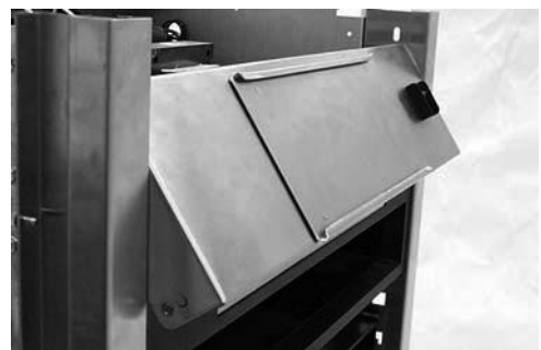
Fig. 3. Removing front fascia.
