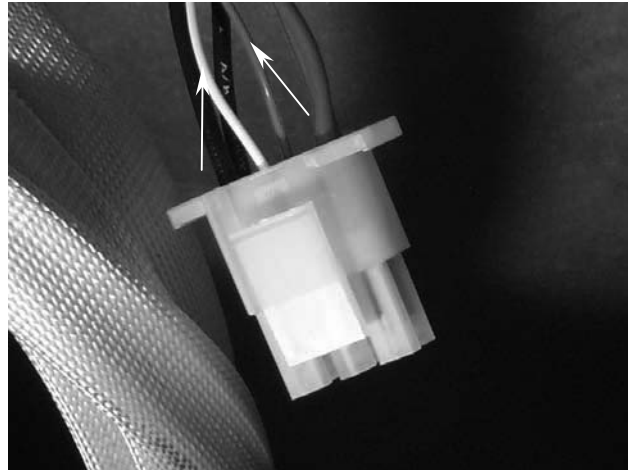
Using a pin-pusher, remove two high-limit wires (arrows) from connector.
