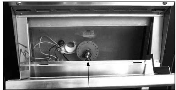
Setscrews hold the knob and dial plate to the thermostat. Use an allen wrench to remove both.
