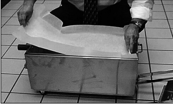
Place sheet of filter paper over the pan, allowing it to drape over the edges.
