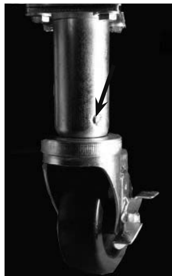
Arrow points to setscrew on front caster.
