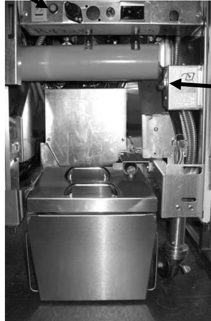
Melting unit power switch
