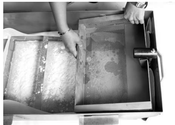
Crumb screen properly placed.
