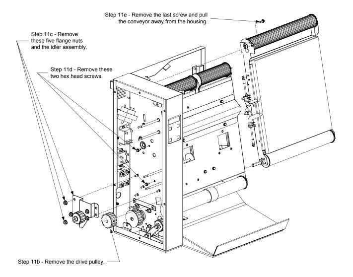
f. Reinstall the conveyor assembly by reversing the steps performed, being sure to reattach the two ground wires with the lower of the two hex head screws removed in Step 11d.
