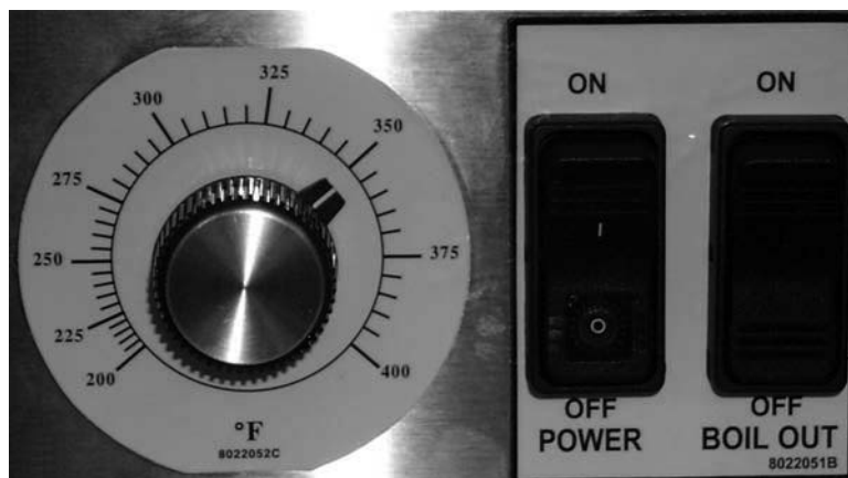
Electronic thermostat controller with power switch and boil-out option.
