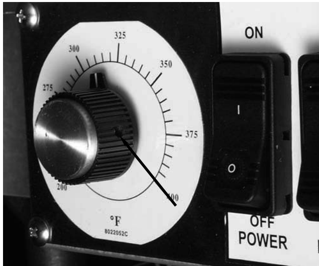
Control knob setscrew location (arrow – counter-set in knob).
