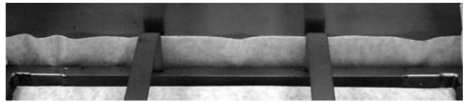
Ensure filter paper overlaps two inches on all sides and is evenly distributed under the hold-down ring.
