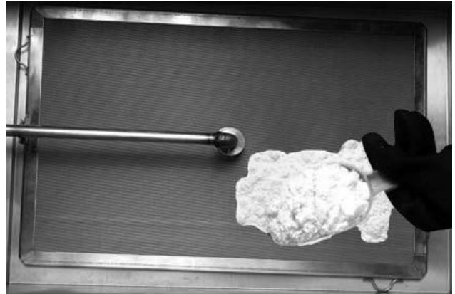
Applying filter powder to filter-leaf.
