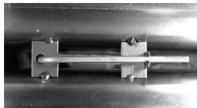
Typical high-limit/sensor probe locations and mounting hardware.
