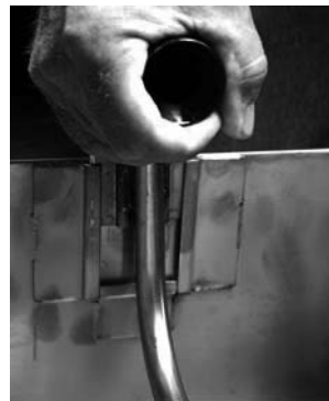
Carefully remove the filter leaf assembly.
