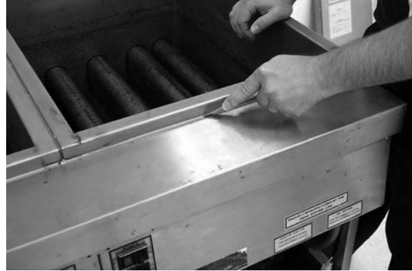
Cutting frypot seal prior to frypot removal.
