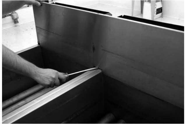
Removing flue cap.
