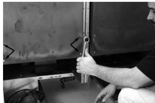
Removing bolts (arrows) securing flue to frypot.
