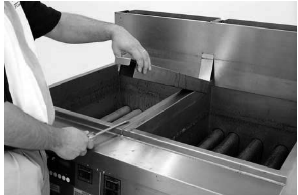
Removing capping strip.
