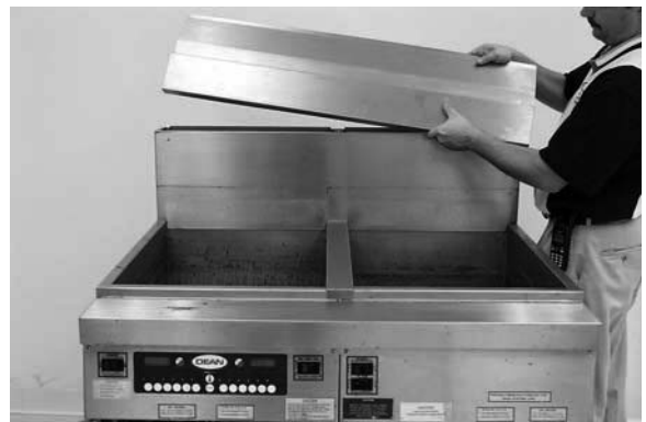
Removing the flue cap.
