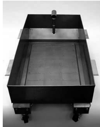
Cleaned support grid in place.
