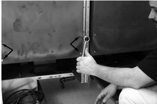
Removing bolts (arrows) securing flue to cookpot.
