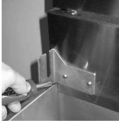
Removing flue cap.
