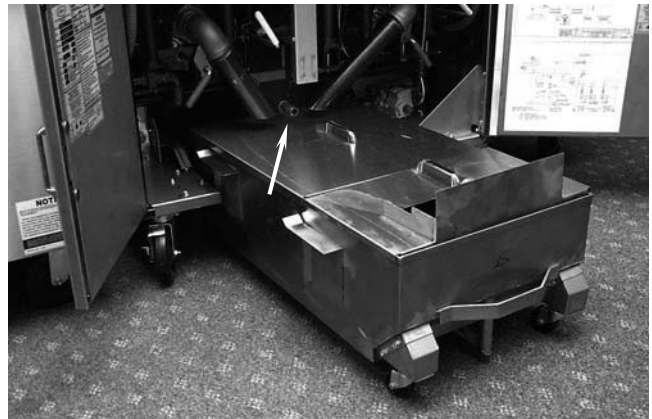
Crumb screen placement in filter pan.
