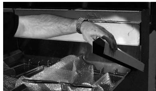
Figure 7. Install joiner strip(s) after fryers are connected.
