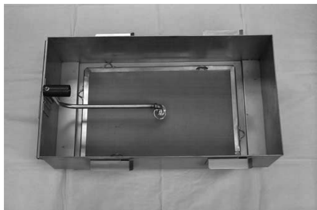
Filter leaf properly positioned in filter pan.
