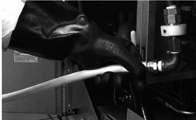
Hose/wand disconnect properly connected to disconnect valve in fryer cabinet (orientation of disconnect may vary according to system).
