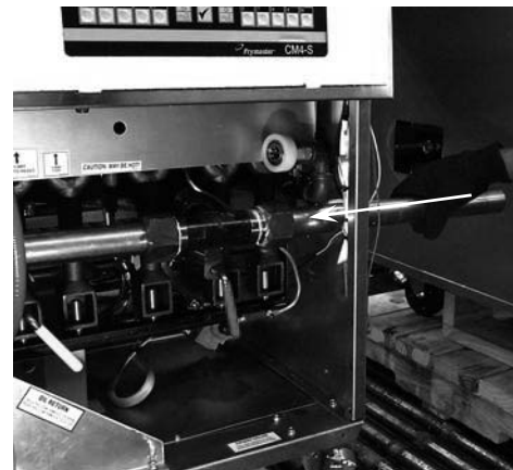
Figure 3. Insert drainpipe section into fryer drain-tee before pushing fryers together (arrow). Do this as required for all cabinets being assembled.
