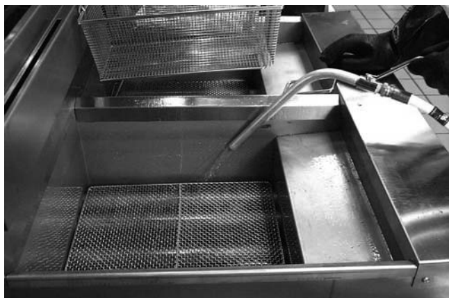
Use the wand to rinse debris from the frypot into the filter pan. Maintain a firm grip on the wand handle at all times.
