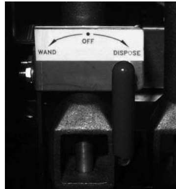
After the hose wand end is properly positioned in the frypot, activate the filter pump by turning the blue handle to "WAND" (where applicable).
