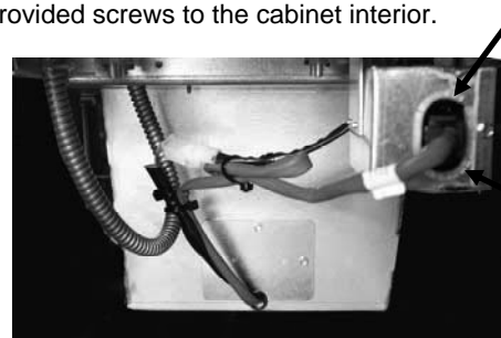
Figure 3: Plug the black connector into the utility box as shown. A separate harness with a white plug, if present, is NOT used.
