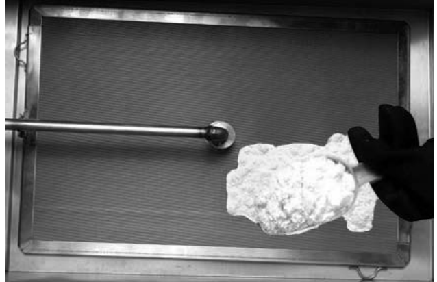
Applying filter powder to filter-leaf.
