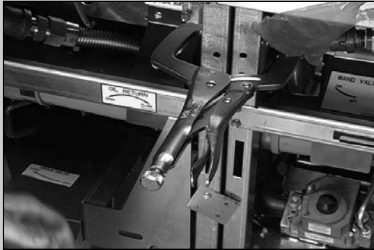
Figure 5: Clamp the fryers together to facilitate mounting securing brackets.
