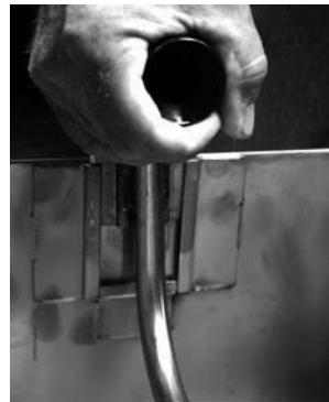
Carefully remove the filter leaf assembly.
