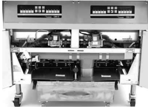
Pull out on the handle to remove the filter pan.
