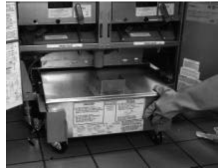
Fig: 12-1 Removing filter pan prior to cleaning.
