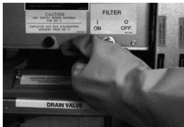
Fig: 12-17 The filter pump moves oil from the drain pan to the frypot.
