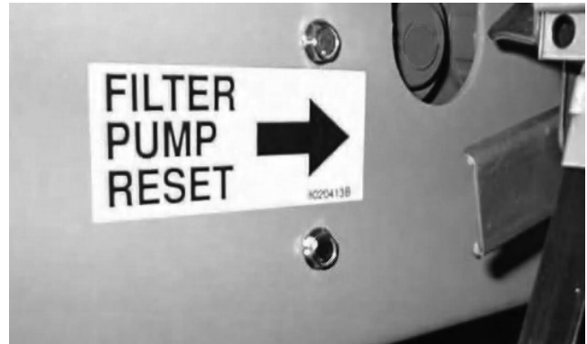
Reset switch location: Old-style FPIII
