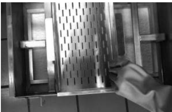
Fig: 12-2 Removing crumb basket.
