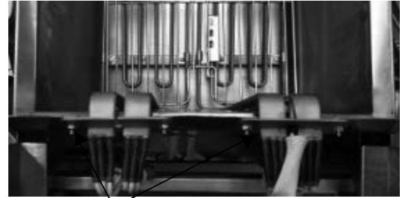
Fig: 10-16 Mounting hardware on fixed-element sub fryer.
