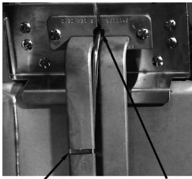
Secure probe to element with metal wire-wrap
