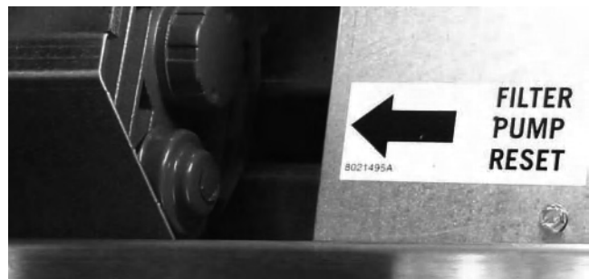
Reset switch location: New-style FP111
