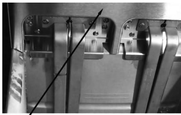
Tilt housing cover in place
