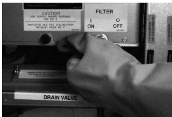
Fig: 12-17 The filter pump moves oil from the drain pan to the frypot.
