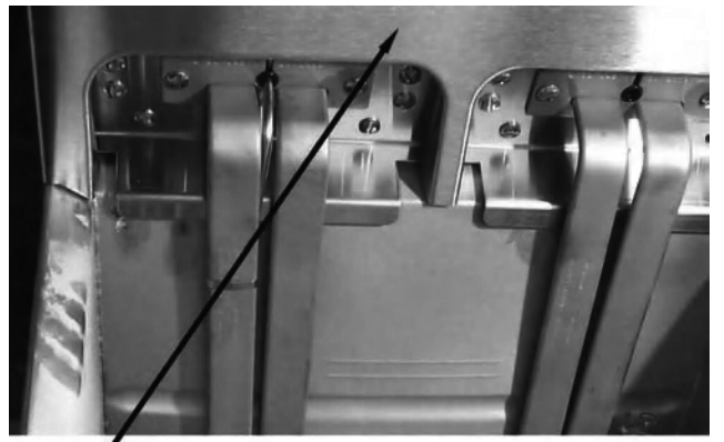
Tilt housing cover in place
